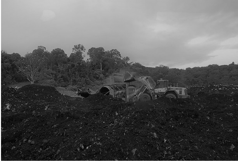
Figure 7. Composting tumbler in operation at Lismore. Photograph: Peter Booth
